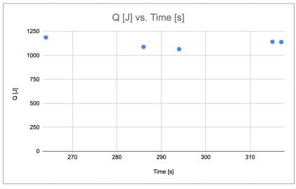
To collect the data for heat gained through conduction illustrated in the graph above we measured initial water temperature, set the kettle to a target temperature, measured elapsed time, then measured final temperature. The heat gained through conduction seen here is much larger than the heat losses due to convection and radiation.
