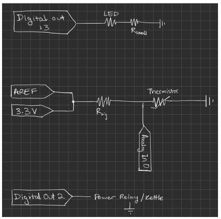
After calibrating our thermistor and ensuring it read roughly the same temperature as provided thermometers, we wrote a simple control loop. It would turn the kettle and LED (as an indicator) on if the thermistor reading was below a certain threshold, and switch it off once it crossed the threshold. We tested it for different target temperatures, keeping volume constant at 5 cups. The graphs are shown below.
