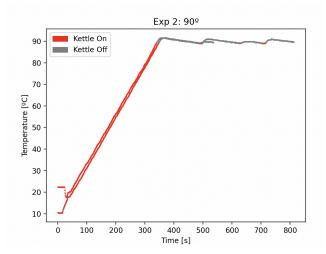
Slightly undershooting to the target helped the temperature stay within about 1 degree of the target. Our final code can be found in the Appendix.
